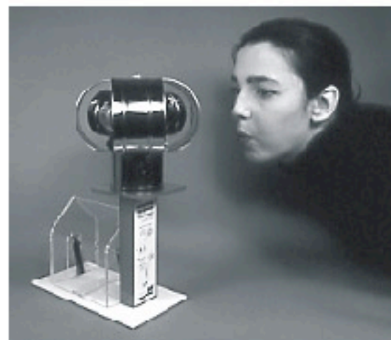
Figure 2: With Vacu-Stack® removed, action is reversed. Oncoming wind deflects Flow Meter Vane away from chimney and towards living space.
